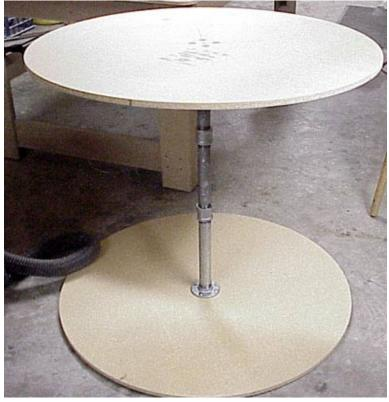
Insert the 1" pipe into the 1 1/4" diameter pipe as shown on the left.
