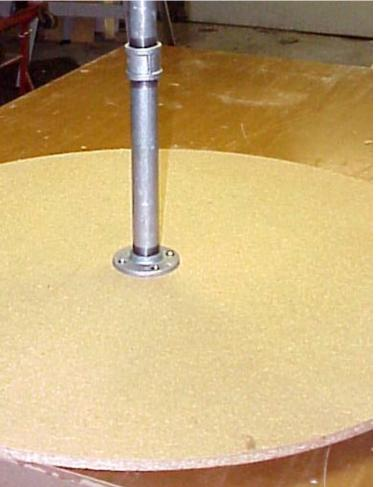
Turn disks over and screw threaded flanges in place with 1/4-20 screws.
