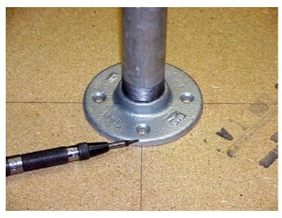
Before cutting disks find the center point of the 48" x 48" square by drawing lines from corner to corner. Place threaded flange on layout lines and line up holes. Use a center punch or marker to mark hole locations. Drill 1/8" deep recessed holes with a 3/4" diameter forstner bit at the indicated points.
